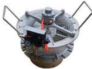
Air Driven Turbine Fans
